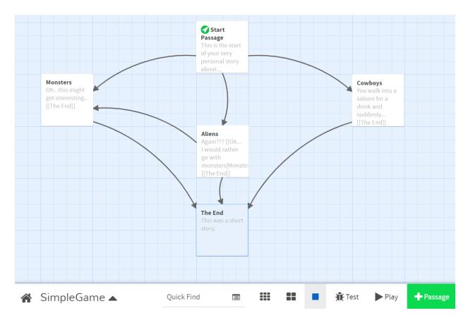
The screenshot shows a simple interactive story in the editor's "Passages View". The story is created directly in the web browser. To create a story, the developer creates different passages, which can be described as different parts of the story. These passages can be connected through links. By clicking on a link, the player is then redirected to a different passage. Often, this is used to generate a choice for the player.
